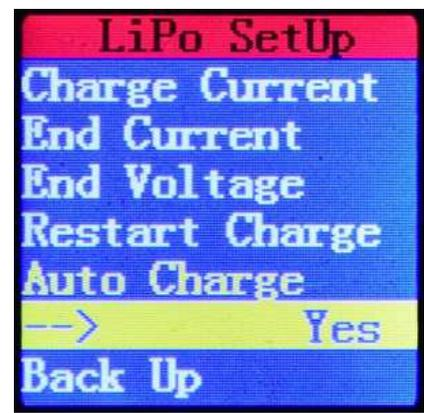
5. Press knob shortly can choose Battery type; press again on Battery type such as LiPo can enter into LiPo charge setup interface. Here, you can setup cell count, charge current, charge terminal current, and charge terminal voltage per cell, and then press knob for 3 seconds start charging.
